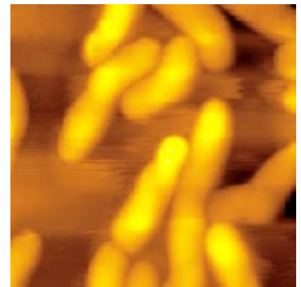
Figure 2. MAC Mode AFM image of living Rhodospseudomonas palustris bacteria immobilized on a gelatin-coated mica surface and imaged in liquid.
