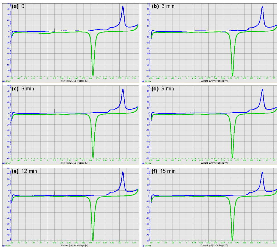
Figure 2. Continuous cyclic voltammograms in 21 minutes of purge from ~5% oxygen concentration.
