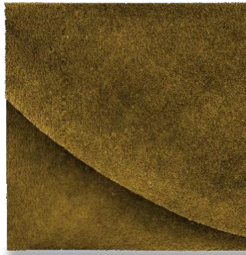
Figure 3. 15 x 15 microns 3D AFM image of the DNA microarray shows the contrast between a probe element and the surrounding silanized glass substrate (lower left).
