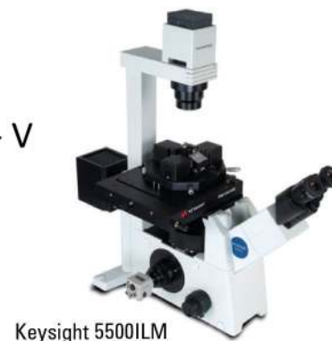
Figure 1. Illustration of Current sensing AFM combined with external illumination for the characterization of photovoltaic materials. Laser illumination could be applied from above the sample as indicated by laser 1, or from below the sample (laser 2) when combined with an inverted optical microscope (as shown by the picture of the Keysight 5500ILM system).
