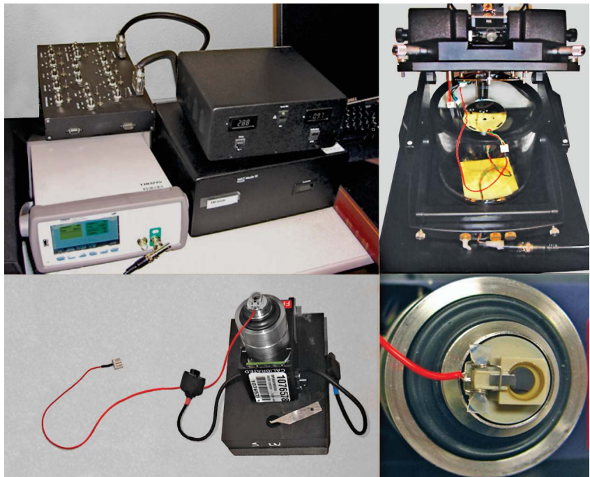
Figure 6. Photos showing the hardware components for high voltage PFM, particularly the modified nosecone with electric lead to connect to the output of the high voltage amplifier.
